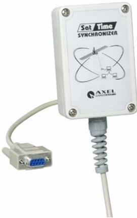
The GPS module receives data from various satellites belonging to the Global Positioning System (GPS), a satellite-based locating and navigating system that allows a user to determine his exact position on earth.
