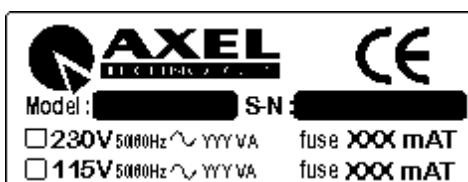
If, for some reason, the unit is to be operated at a mains input voltage which is different to that as supplied, you need to switch the voltage selector on the right side of the unit. You also need to replace the AC main fuse, according to information provided on the external label or on the Technical Specifications table at the end of this user manual.
