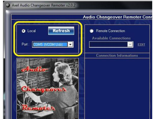
Clicking the Connect key, the Audio Changeover Remoter enters into communication with Genius D, and all the information in the memory of the device, the status and operation of the same will be displayed. The management panel changes format and offers all the commands necessary for putting into operation of the device. The various controls are explained in detail in the next few chapters.
