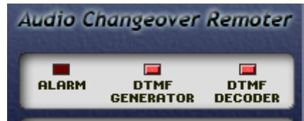
**DTMF Generator:** this red indication represents the capacity of Genius D to generate a series of DTMF Tones, with user-customisable strings. The indication only represents the ability of Genius D to generate DTMF tones, and not that Genius D, when the DTMF GENERATOR led is lit, is generating DTMF tones.
