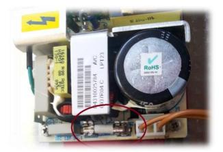
c. Replace the fuse located at the internal position – Power supply Type-2
