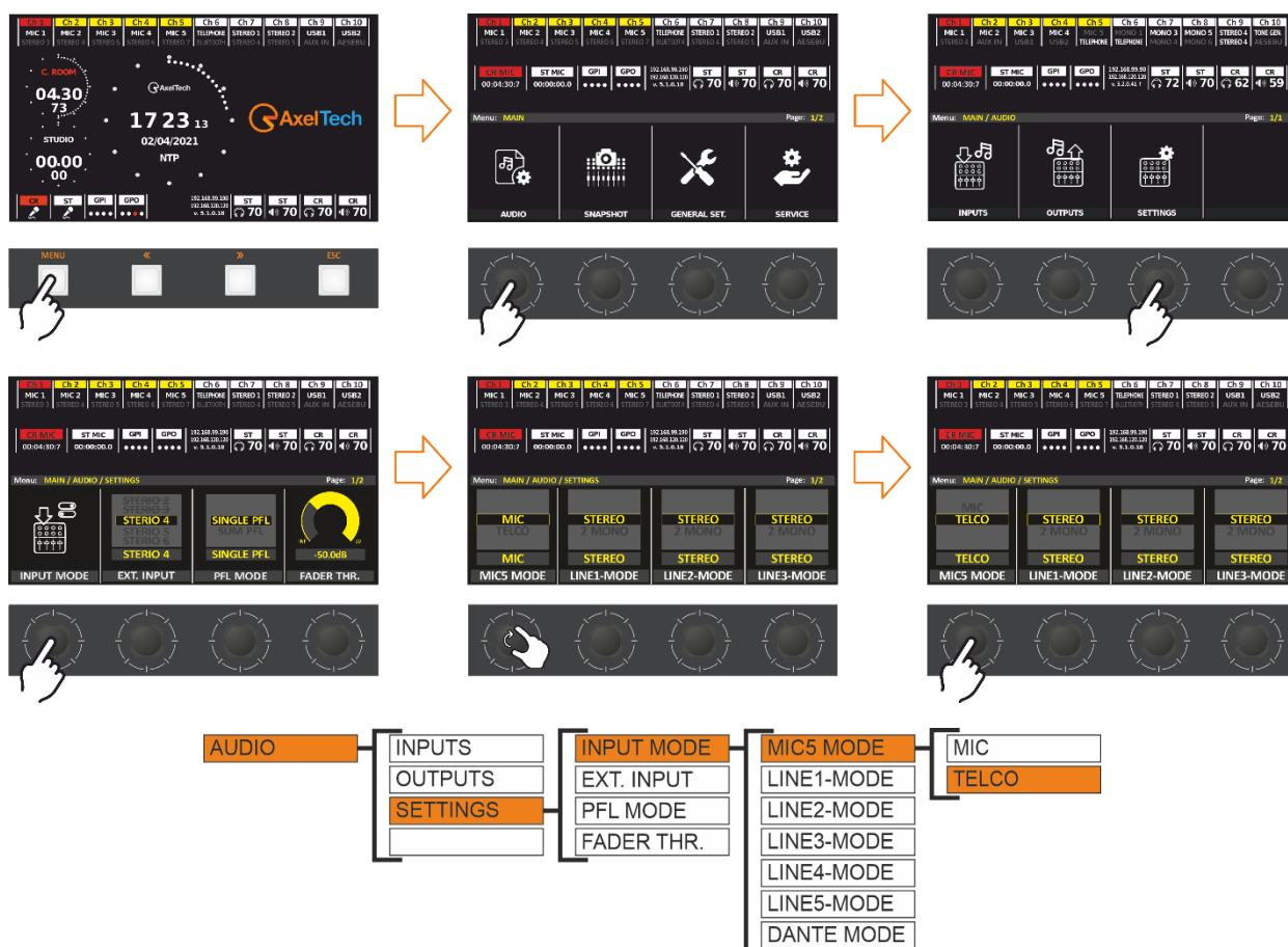
When you change the **MIC-5** to **TELCO MODE**, the **MIC-5** in the input microphones setting will show in a grey color to indicate **MIC-5** is inactive.
