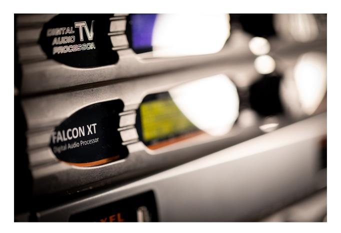
The hardware bypass circuit is always included to ensure audio presence and audio programs continuity. Falcon XT meets the most demanding broadcasters with extremely sophisticated audio features and high standards level: 5-band control compression, dual-band power AGC, three-band EQ and Brightness control.
